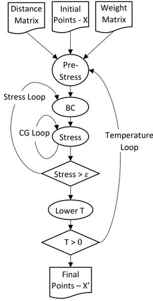
Fig. 4. Multidimensional Scaling algorithm with Deterministic Annealing control flow
