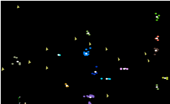
Figure 2. A tiny fragment of clustered space for a full DAVS(1) run. The orange triangles are sponge peaks outside any cluster. The colored hexagons are peaks inside clusters with the white hexagons being determined cluster centers. Each cluster is colored differently. This comes from 241605 peak charge 2 clustering.
