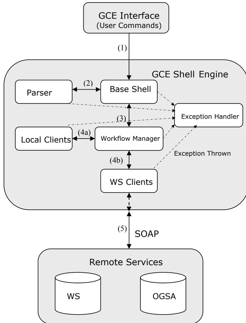
Figure 1: GCE Shell execution steps and block diagram
