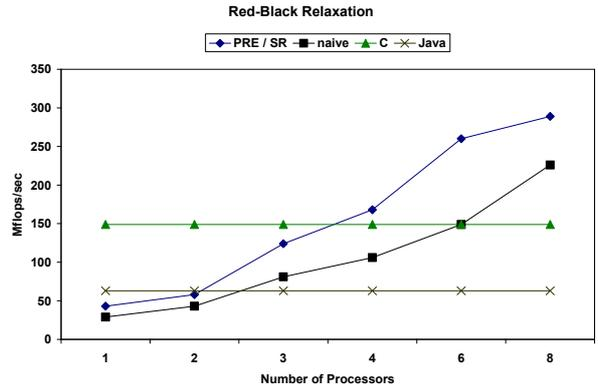
**Figure 6. Laplace Equation with red-black relaxation with size of 512 x 512 on Sun Solaris 9 with 8 UltraSPARC III processors.**
