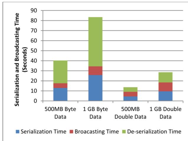
Figure 6. Serialization, Broadcasting and De-serialization
