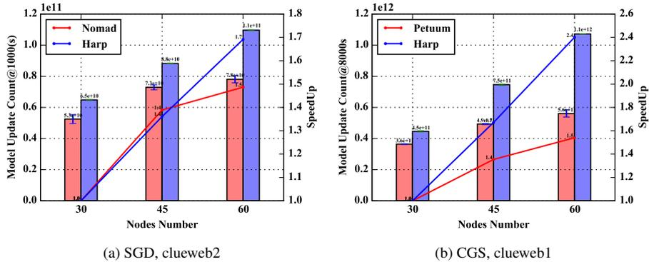
Figure 4. Scaling of SGD and CGS on 30, 45, 60 Xeon E5-2699 v3 Nodes
