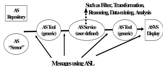
Figure 2: Application Specific Information System architecture for application specific Sensor Filter Grids.
