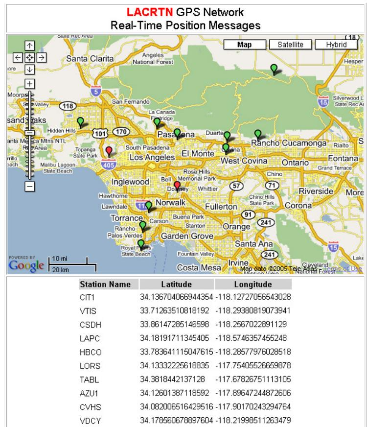
**Figure 3** Google maps are used to display live GPS station feeds, after several filtering steps.
