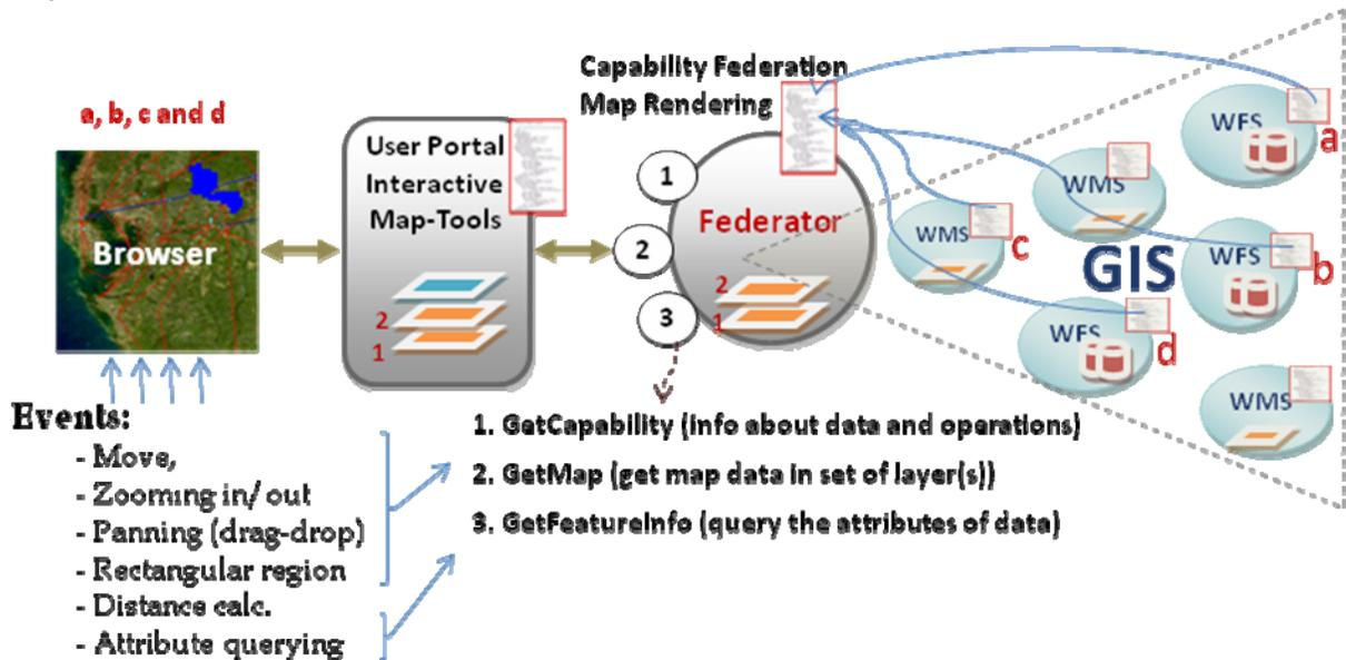
Figure 1: Federated, service-oriented Geographic Information System framework supports decision making over integrated data-views.
