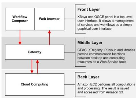
Figure 1. Three-layered BioVLAB-MMIA
