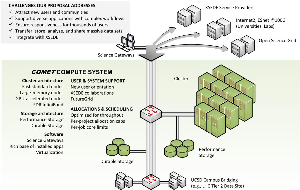
**Figure 1.** High-level view of *Comet* summarizing the architectural features, relationship between main components and how *Comet* will support a diverse community of users with a wide range of compute and data requirements.
